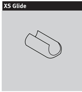
XS Glide 1/8-inch-high glide; polycarbonate in black, fog, clear, and studio white finishes; for use on hard floors or carpet Applicable on: Sayl Chairs
