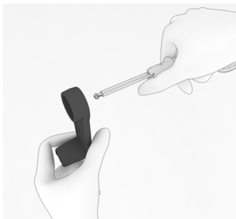
41. Insert new front link into tilt limit control.
