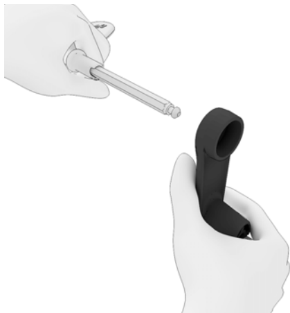
39. Insert new front link into tilt tension control knob.
