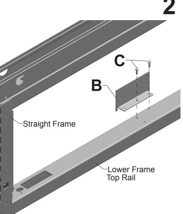
In the case where change of height is created by addition of a Stacking Frame and Off Module Tile must be installed at top of Lower Frame, Support Bracket (B) must be installed on Top Rail of Lower Frame.
