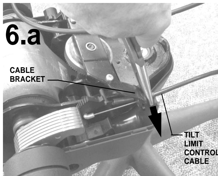
6.a.1 Remove tilt limit control cable by first removing cable from cable bracket with needle nose pliers.
