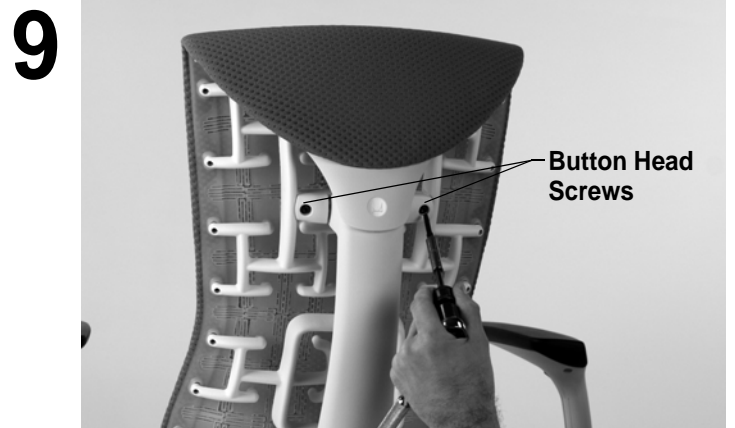
Install 2 Torx Button Head Screws previously removed. Torque screws to 35 in/lbs.
