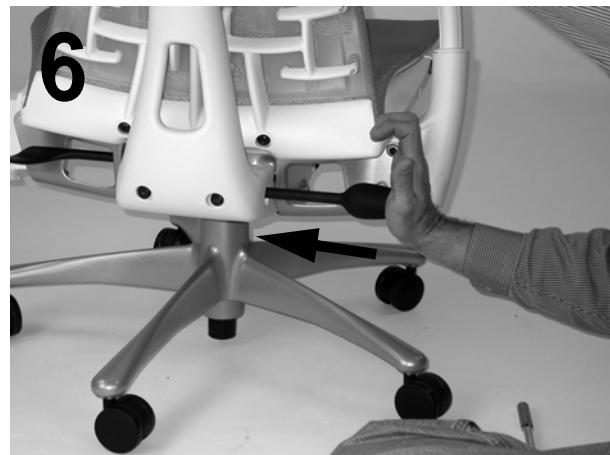
6. Replace back tension adjustment knob by pushing all the way in and then strike with palm of hand until seated. An audible click should be heard.
