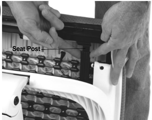
Slide replacement Seat Slide Guide with Spring inside onto Seat Post.
