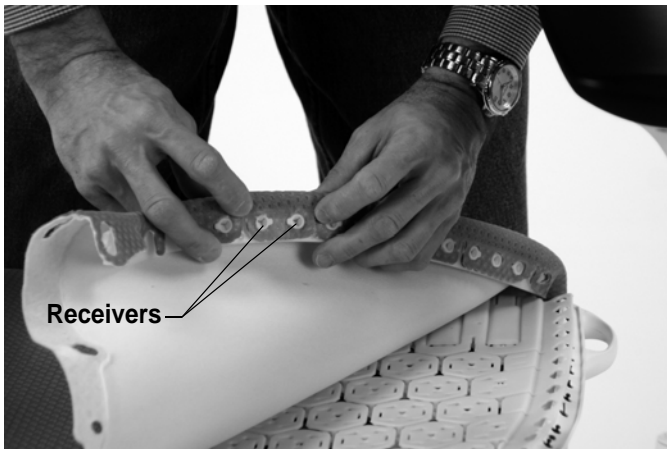
Make sure fabric is captured by Receivers.
