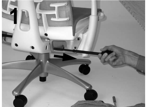
1. Remove back tension adjustment rod by wiggling up and down while pulling out to disengage.
