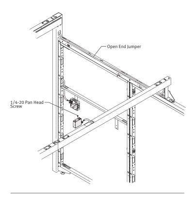
5.2 Disconnect Molex Quick Connector from LED board. Remove end LED Cartridges.
