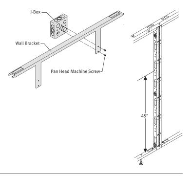
NOTE: The configuration shown is just one example of many. Use same installation processes for all configurations
