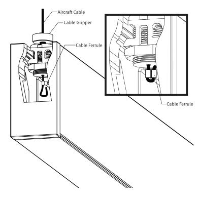
5.4 Secure Power Cord to Aircraft Cable with Plastic Clip. Make final adjustment of cable height by pushing Cable Gripper downward.
