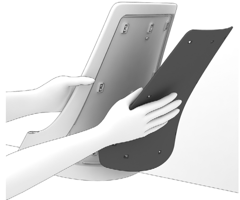
14. Remove fabric plastic back panel.
